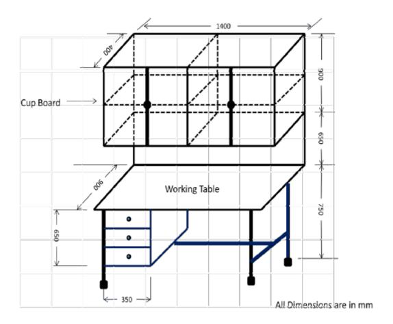
Drawing of Cup Board and Working Table
