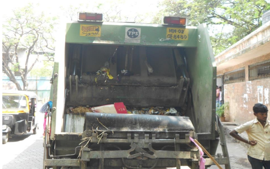
Figure 3.3: Pictorial View of a compactor used for Transportation of MSW in MCGM, Mumbai Region
