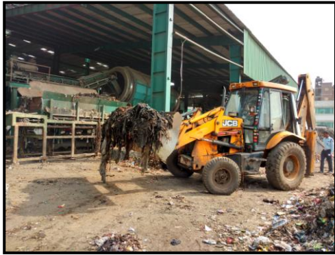
Fig.4 Loading and Separation of plastics from 80mm Trommel/Sieve
