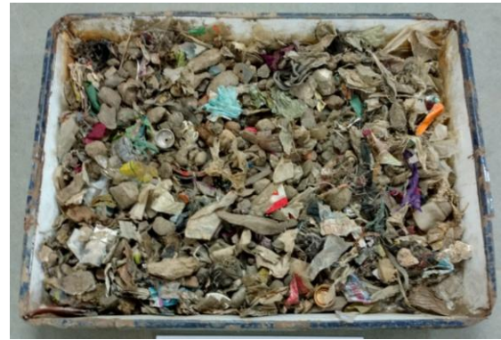
Fig.23 (b) Fraction retained on 16mm sieve after air blowing
