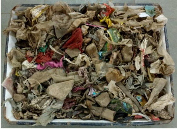
Fig.22 (a) Fraction retained on 37.5mm sieve before air blowing
