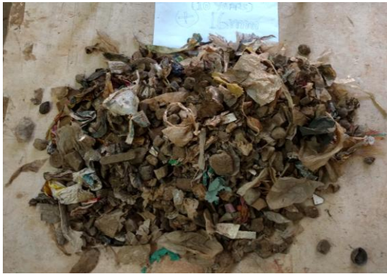
Fig.23 (a) Fraction retained on 16mm sieve before air blowing
