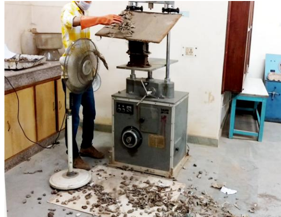
Fig.21:- Experimental setup for segregation of fractions retained on 37.5mm and 16mm
