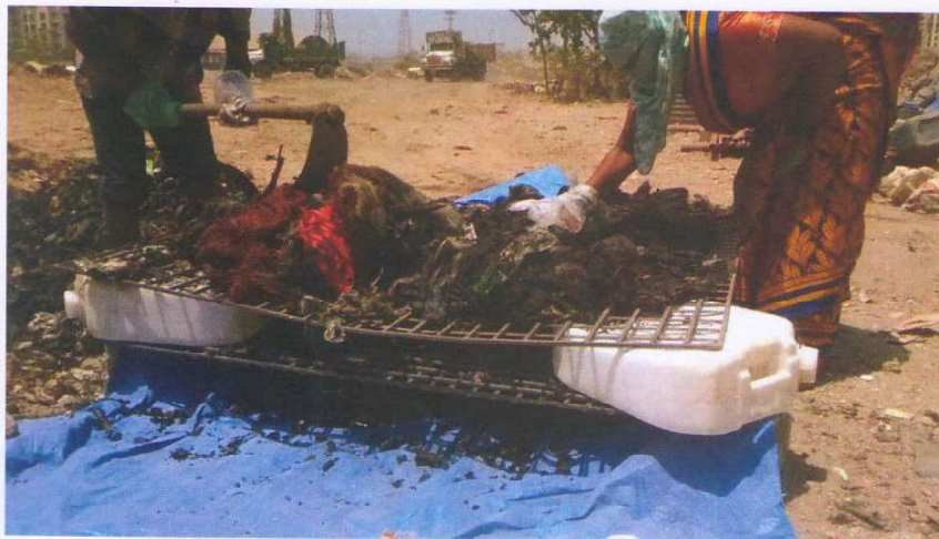
Figure 4. Sieving of the waste materials into different fraction using 50 mm and 20 mm screens place one over the other
