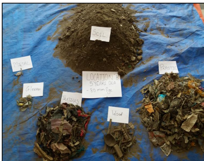
Fig.12 Manual Separation of MSW passing 80mm
