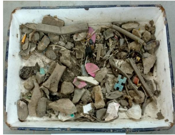
Fig.22 (b) Fraction retained on 37.5mm sieve after air blowing
