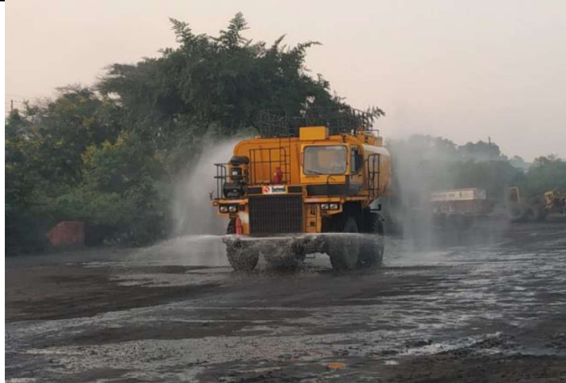
Mobile water cum mist sprinkler
