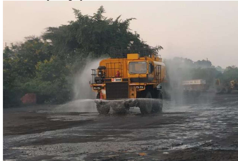
Mobile water sprinkler
