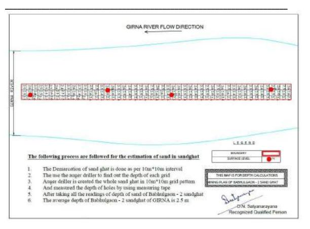
15. Replenishment study of sand in the proposed ghat along with details of methodology, technology used to identify the existing reserve and replenishment of the same.
