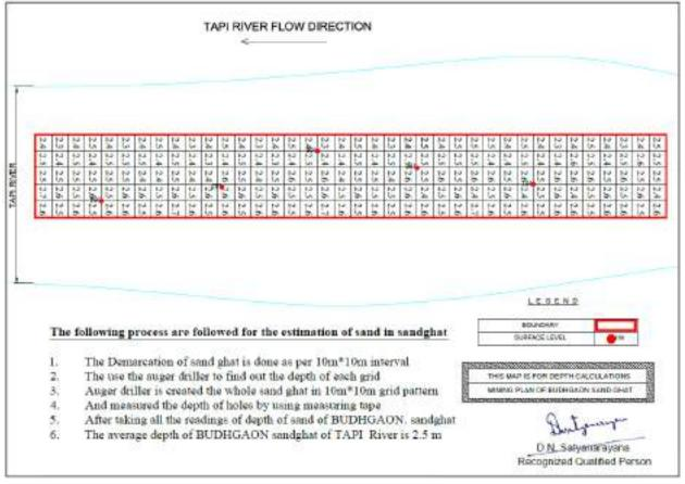
15. Replenishment study of sand in the proposed ghat along with details of methodology, technology used to identify the existing reserve and replenishment of the same.
