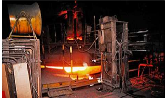
Ladle Furnace Vacuum degasifying
