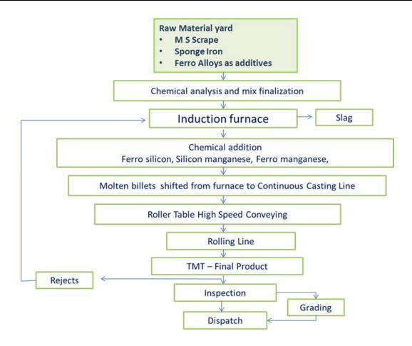
**Figure: Process Flow Chart of the Project**
