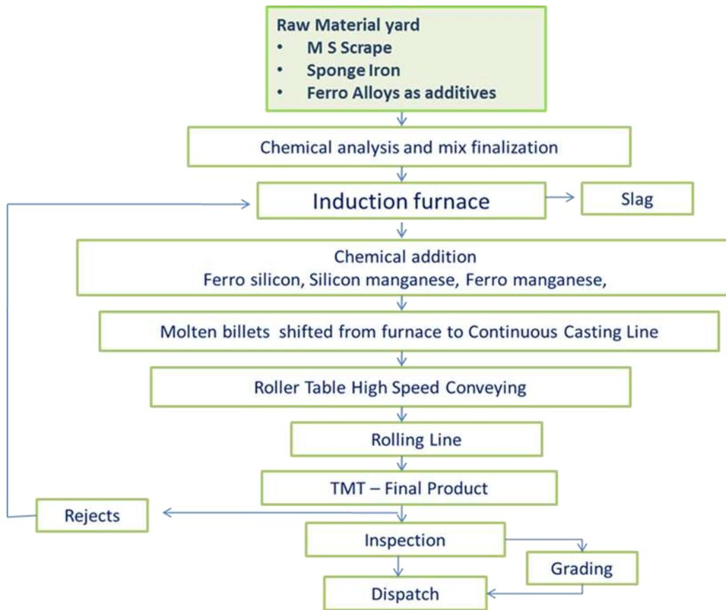
**Figure: Process Flow Chart of the Project**
