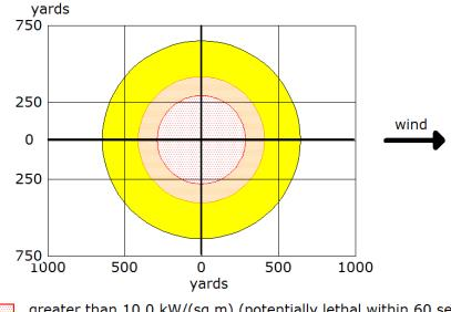
greater than 10.0 kW/(sq m) (potentially lethal within 60 sec) greater than 5.0 kW/(sq m) (2nd degree burns within 60 sec) greater than 2.0 kW/(sq m) (pain within 60 sec)
