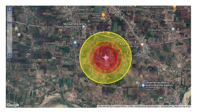
The Thermal radiation from fireball of Ethanol having value of 5 kw/sqm is Vulnerable for second degree burns to all the plant personnel in the radius of 1.1 mile
