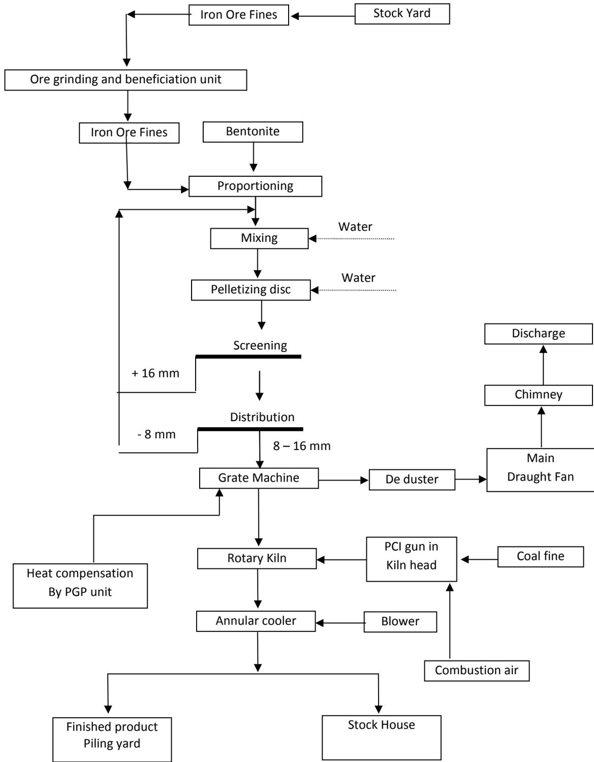
**Flow chart of process of Pellet Plant**
