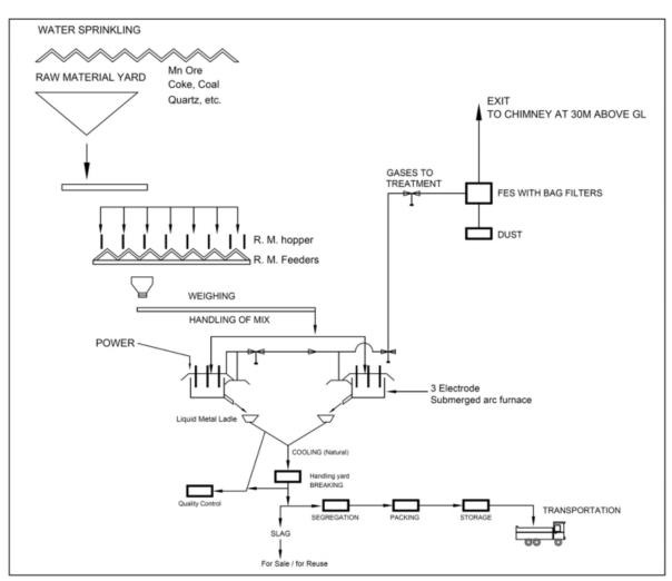
Schematic diagram showing process flow diagram of Ferro Alloys Manufacturing
