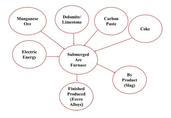
Flow Chart of Ferro Alloys Manufacturing
