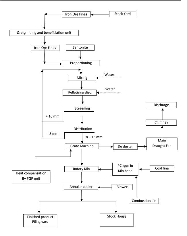
Flow chart of process of Pellet Plant
