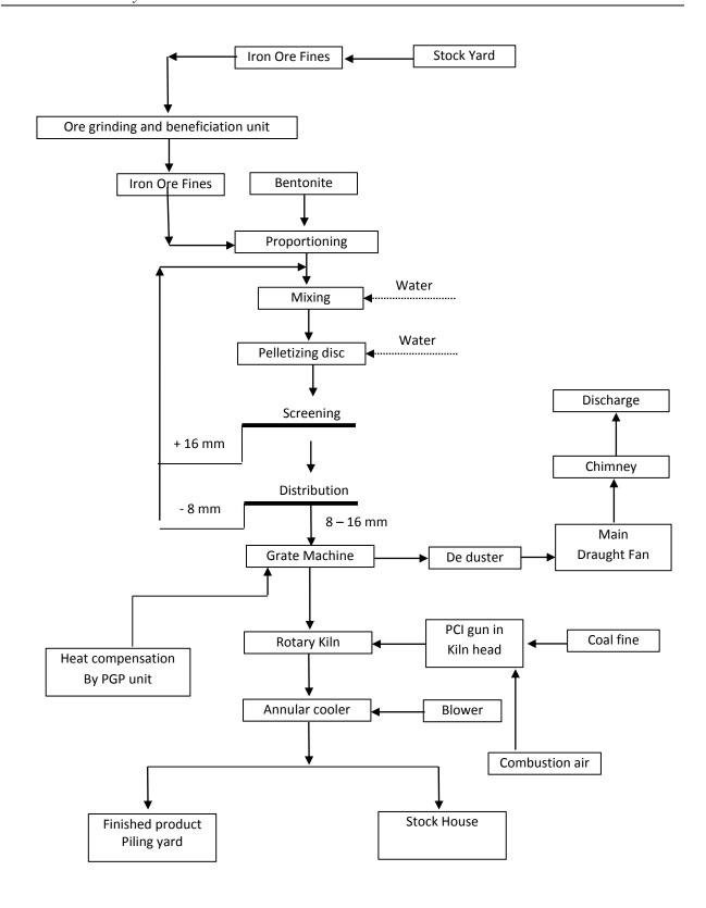
Flow chart of process of Pellet Plant
