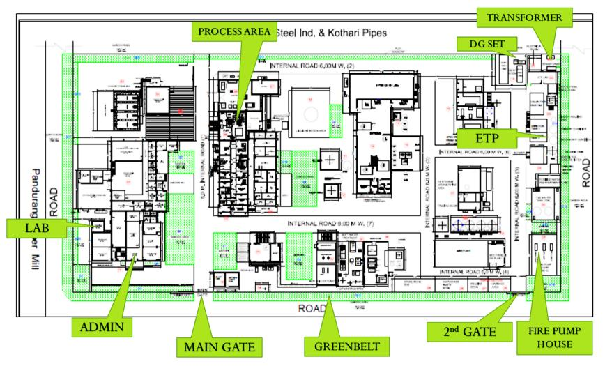
Figure No. 3: Plan layout of Existing Unit
