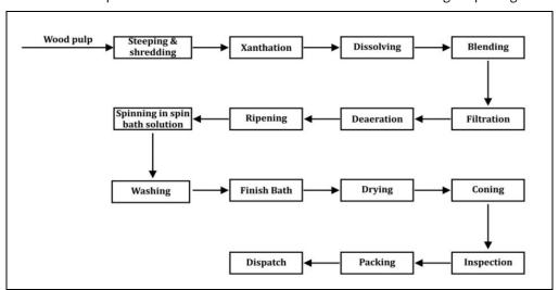
Figure 2: Process Flow Diagram of Viscose Filament Yarn
