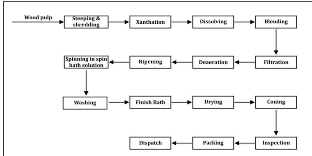
Figure 2: Process Flow Diagram of Viscose Filament Yarn
