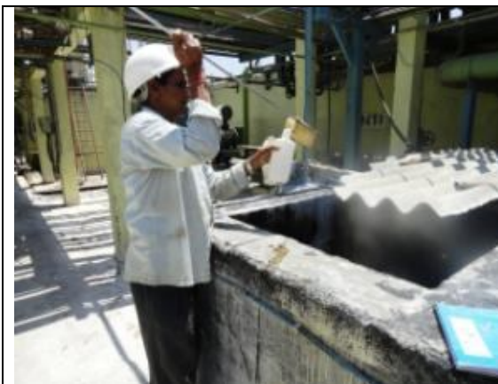
Photo Plate 3.9: Treated Waste Water Sample Collection from ETP
