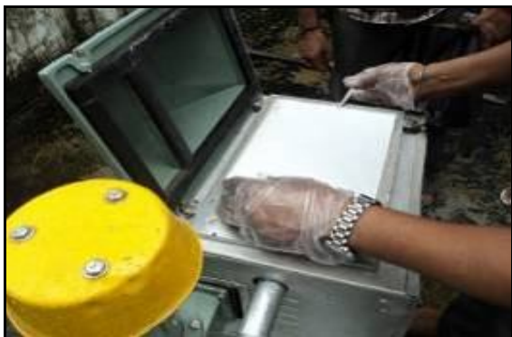
Photo Plate 3.13: Filter paper for monitoring the PM 10 at Valap village
