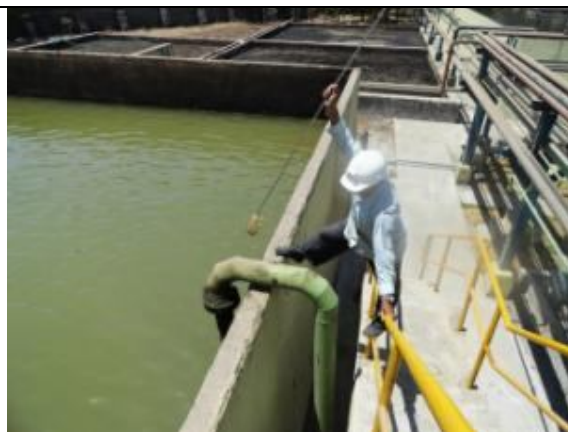
Photo Plate 3.10: Untreated Waste Water Sample Collection from ETP
