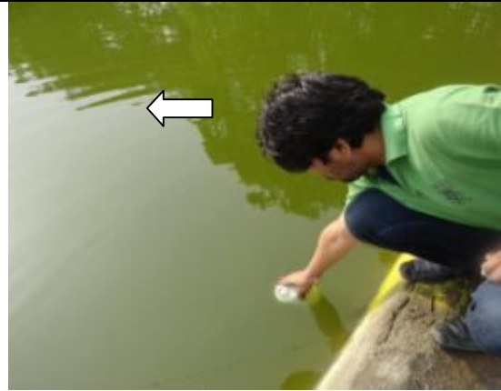
Photo Plate 3.5: Surface Water Sample Collection from Kasardi river
