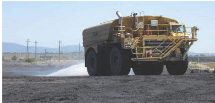
Figure 1 : Road side sprinkling of dust control agents
