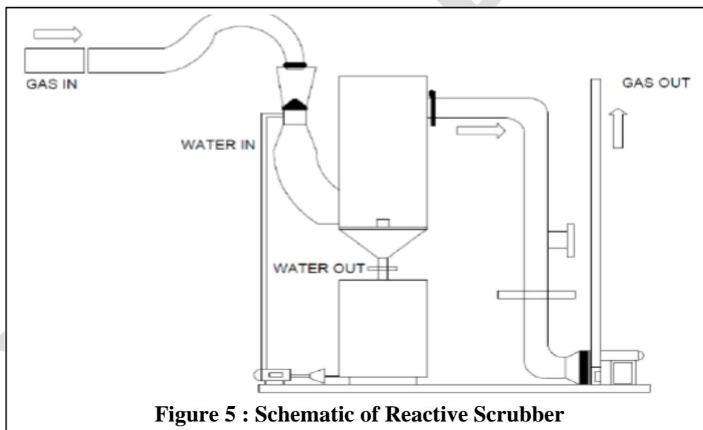
**Figure 5 : Schematic of Reactive Scrubber**
