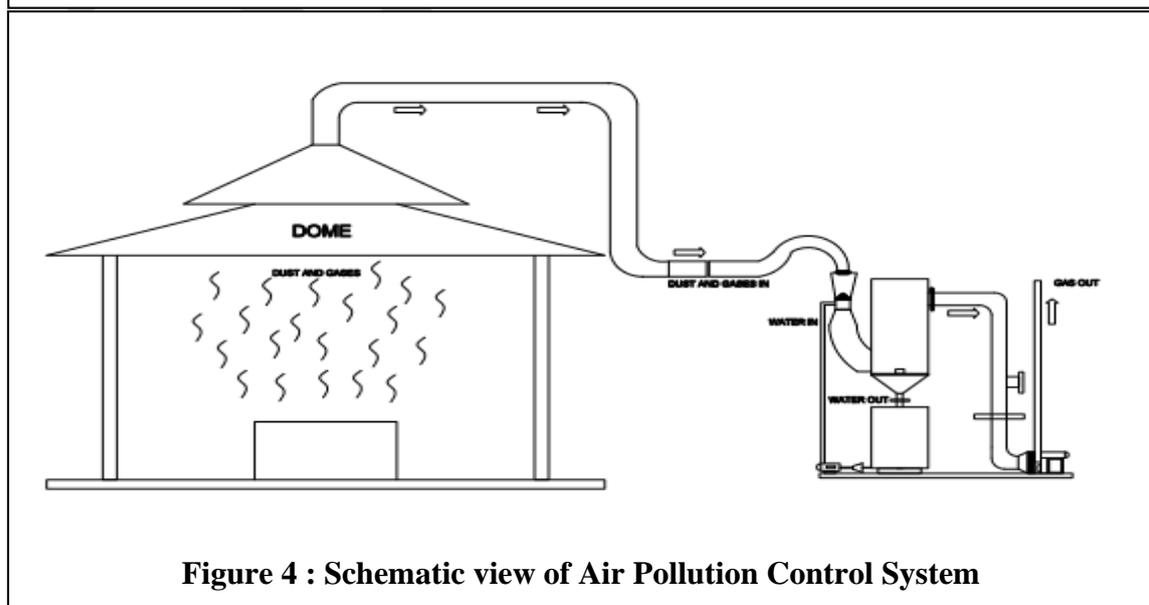
**Figure 4 : Schematic view of Air Pollution Control System**
