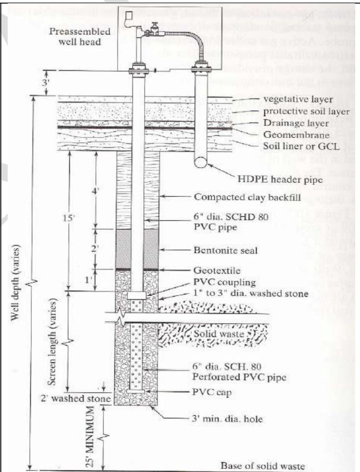
**Typical Design of Passive Vent System**
