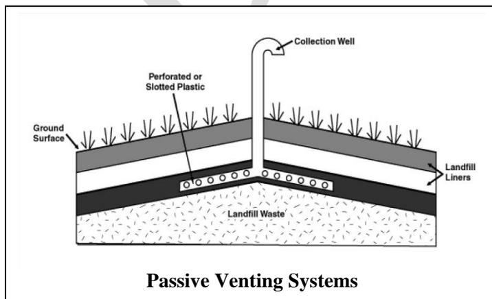
installed during active operation of a landfill or after closure. Passive systems use collection wells, also referred to as extraction wells, to collect landfill gas. The collection wells are typically constructed of perforated or slotted plastic and are installed vertically throughout the landfill to depths ranging from 50% to
