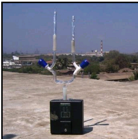
Photograph showing use of ATD tubes in field monitoring
