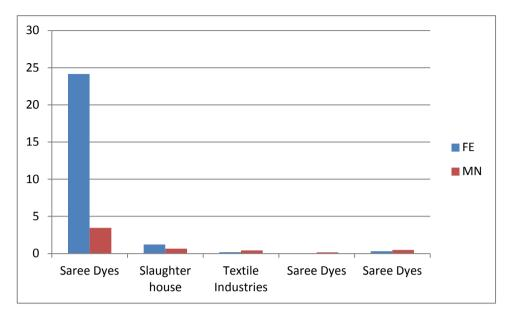
Fig. 3.18: Fe and Mn values (Industrial Effluent affecting Girna)
