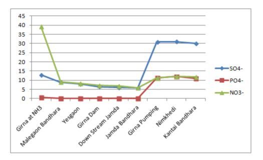
Fig. 3.5: SO4, PO4 and NO3 values (Surface water Girna)
