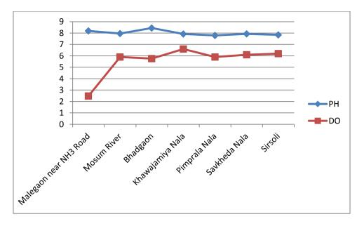
Fig. 3.11: pH and DO values (Domestic waste water Girna)
