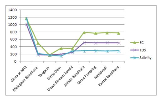
Fig. 3.2: EC, TDS and salinity (Surface water Girna)
