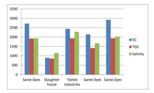
Fig. 3.15: EC, TDS and Salinity values (Industrial Effluent affecting Girna)
