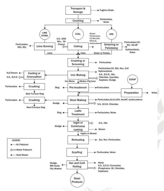
From the above diagram, it is clear that pelletization is a definite source of pollution. It generates Particulates, CO, SO<sub>2</sub>, NO<sub>2</sub>, HF, Hydrocarbons and noise. All these pollutants have serious impacts on the environment. Thus, undoubtedly, it requires greater checks and restrictions to ensure prevention of pollution.
